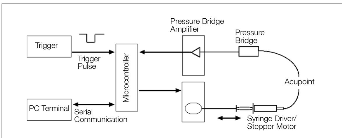
1 Volt peak-to-peak trigger pulse can be provided from any source. This system is configured for 2 sources; 1. Manual push button operation for use in the PI validation study; 2. Automatically from a square wave pulse delivered from a Siemens Magnetom (Siemens, Erlangen, Germany) MR scan system.
